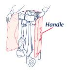
**2** Lift *Floor Handle*, rotate counterclockwise to unlock
